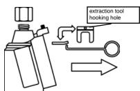
Extract the clip putting the extraction tool (KM/3062) in the hole of the security clip then pull hard to extract the clip.
